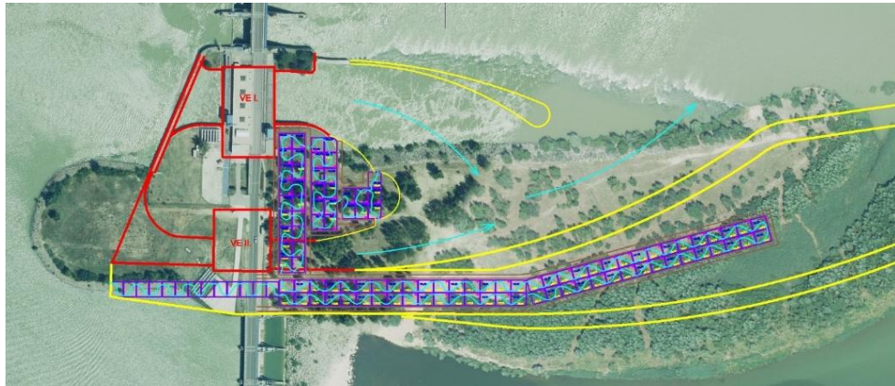
Technical solutions – fishpass for sturgeon species Čunovo dam (incl. Huso huso )
